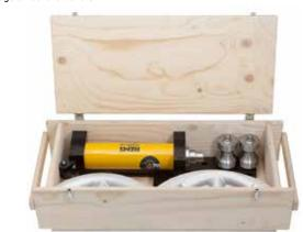
**REMS Python Set.** Oil-hydraulic pipe bender for dimensionally accurate bending of pipes up to  $90^\circ$ . Steel pipes EN 10255 Ø % –  $2^\circ$ , multilayer composite tubes Ø 32 – 75 mm. Drive unit with back former supports, upper back former support with laterally adjustable back former support bearing plate, 2 back formers, bending formers St or V. In sturdy carrying case.
