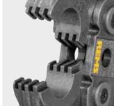
Pressing tongs with teeth prevent formation of burr on the pressfitting. Patent EP 2 027 971
