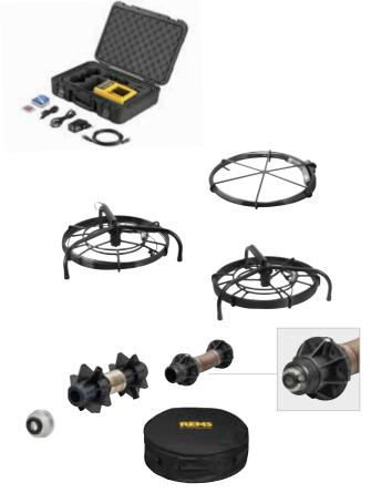
Mobile, handy camera inspection system for inexpensive inspection and damage analysis of pipes, drains, chimneys and other hollow cavities. Self-levelling camera. Transmitter for localising camera heads. Electronic metering. Also for inspection after pipe cleaning work and for acceptance of new installations or repairs. Documentation of pictures and videos with voice recording on SD card. For battery and corded operation.
