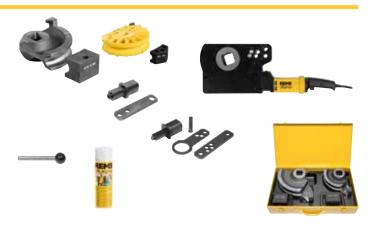
Universal, mobile electric tool for cold bending of pipes up to 180°. Can be used anywhere, without vice. For trade and industry. For the building site and the workshop. Li-lon 22 V Technology. For battery and corded operation.
